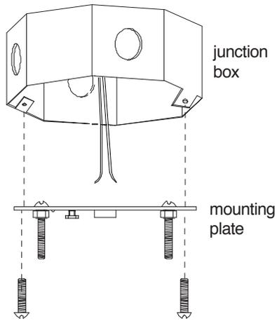
Shut off the main electrical supply from the main fuse box/circuit breaker. Carefully unpack all fixture parts and hardware. Lay items out on a clear workspace. Place the **mounting plate** over the center of the ceiling junction box. Align holes in mounting plate with holes in junction box and attach with 2 **mounting bolts**. Secure bolts with a **phillips head screwdriver**.
