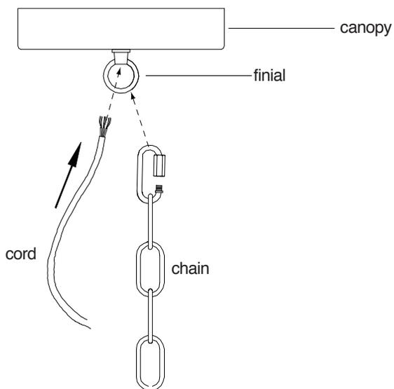
Insert cut end of **cord** into corresponding hole of **finial** and **canopy** as shown. Hook and fasten **chain** to **finial** as shown.
