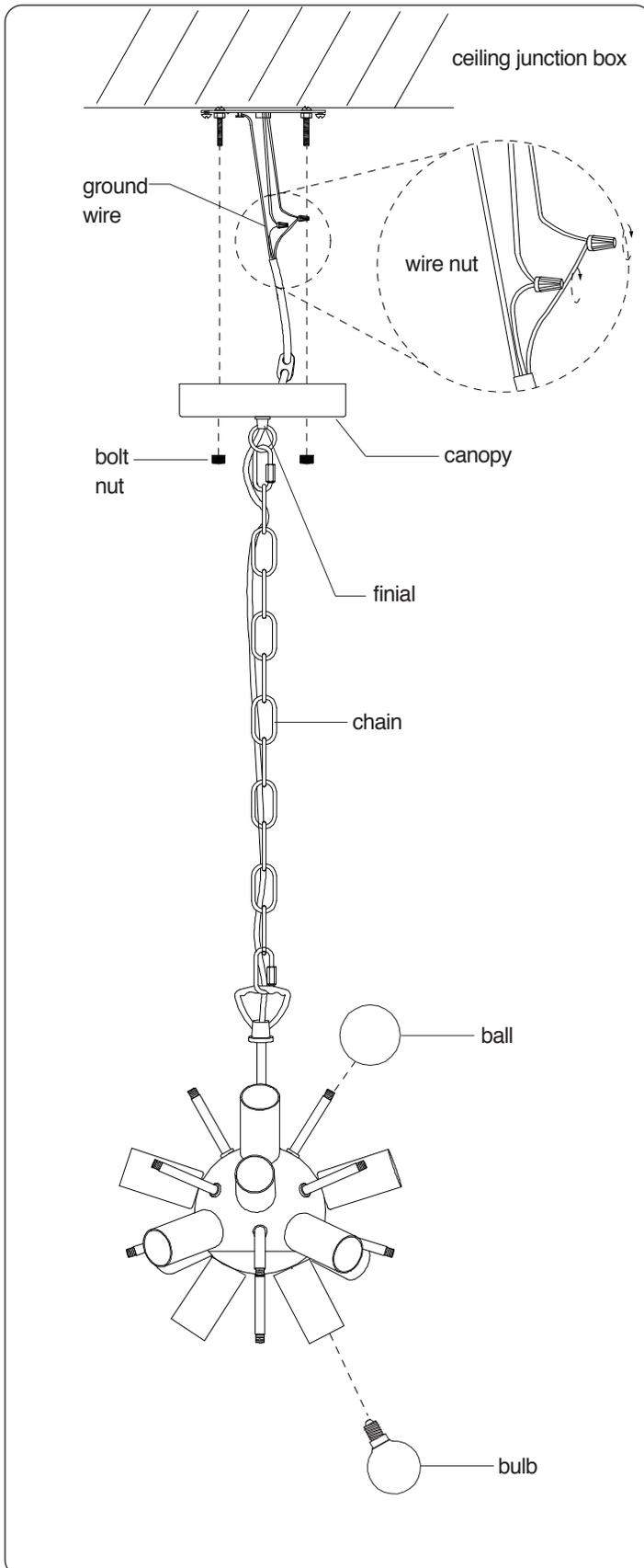
1) Gently pull wiring down from ceiling junction box and allow it to hang
