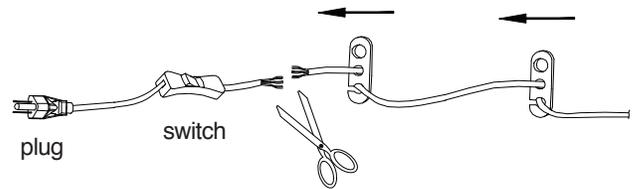
Carefully cut pre-attached plug and switch off **cord** as shown. Discard plug and switch.
